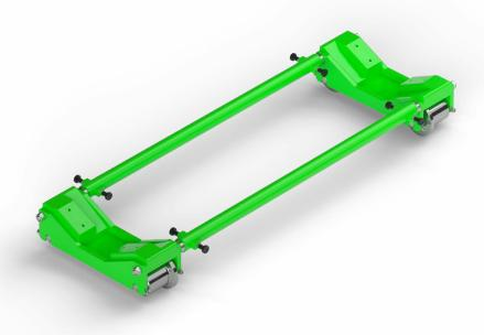
To be fitted with SAMS' rerailing kits, the lorry is used in the event of a derailment with bogies or axles out of services. Withstanding up to 30 tons, it allows the damaged vehicle to be brought back to the depot.
