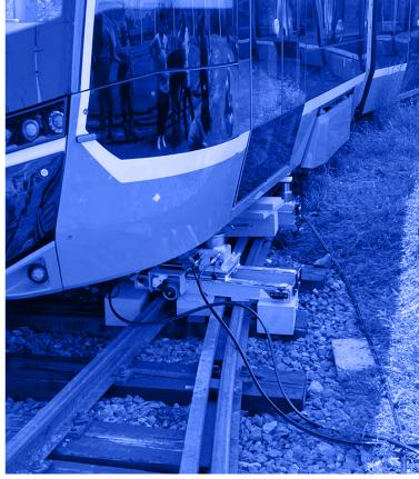
Classic derailment situation without any difficulty of terrain or height. Vehicle derailed less than 500 mm from the rails Tram with re-railing side slots, at a significant height.
